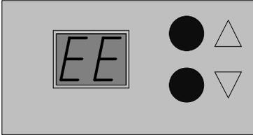
Any error message indicates problems that must be repaired. Some errors may leave the LP600 functional in manual mode only.
