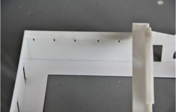
Glue on the small top piece between the top wall pieces, then glue on the two roof support strips for the rear roof. Mount it a strip width below the top edge.
