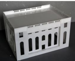
Glue on the top pieces, starting with the long sides, then glue in the roof.
