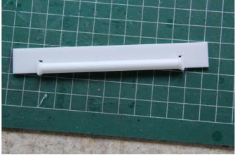
Use the column tool to cut the styrene tubes to the correct length, them use it to place the trim rings and squares and glue them on. The rings and squares with the "flat" side go on the 8 end columns (see picture on the next page).
