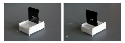
Remove the protective paper from the clear acrylic and glue it to the inside of the crossbar, then glue the black window piece onto the clear, resting on top of the crossbar as shown.
