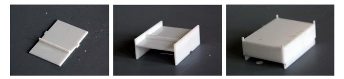
Glue the crossbar to the base as shown. Then glue the sides on, and finally the bottom and the end pieces.
