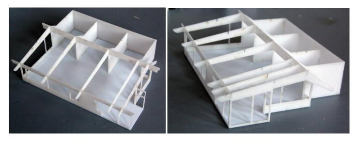
Glue on the rear wall, fit the roof top beam in the slots and glue. Mount the last right side wall piece.
