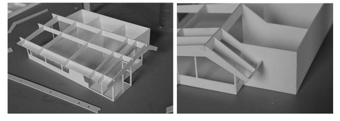
Mount the long front and right rear fascia board fitting the small tabs into the slots
