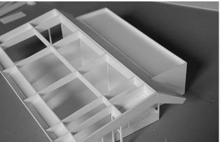
Mount the narrow roof part and the flat roof on the kitchen section.
