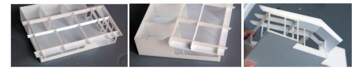
Glue on the eave boards along the front, the left side, and the 2 small pieces on the right side. Mount the middle support beam in the slots and glue.
