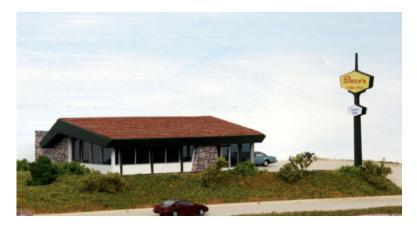
This kit includes all building parts milled in white styrene plastic, clear window glazing, self-adhesive laser cut shingle roofing, and self adhesive logo decals. All parts fit together but may need light sanding in joints for cosmetic reasons. The model needs painting.
