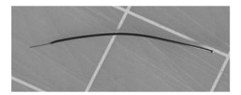
Cut the black wire into 8  $1\frac{1}{2}$ " (38 mm) pieces and strip 0.2" (5mm) Make a 90 degree bend in the bare wire and mount it in the hole in the nozzle opening. Bend the wire to fit and attach the other end to the top of the side with a small drop of CA glue.
