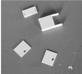
Glue the front piece on so the small hole is to the right when viewed from the front. Glue on the other side and front piece.
