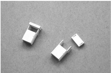
Glue the front piece on so the small hole is to the right when viewed from the front. Glue on the other side and front piece.
