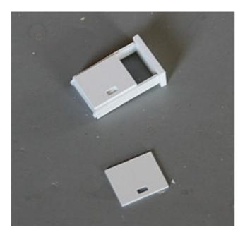
Glue the top onto the pump, fitting the sides into the slots in the top.
