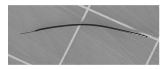
Cut the black wire into 8  $1\frac{1}{2}$ " (38 mm) pieces and strip 0.2" (5mm) Make a 90 degree bend in the bare wire and mount it in the hole in the nozzle opening. Bend the wire to fit and attach the other end to the top of the side with a small drop of CA glue.
