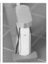
Mount the decal on the pump top, making the seam in the middle of the half-circle. Choose the side, which will be the least visible. The decal may work itself loose (because of the bend), so secure the seam with a small drop of yellow paint.
