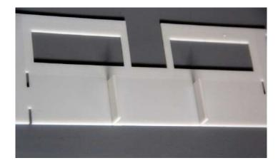
Glue the two front overhang supports to the front wall.
