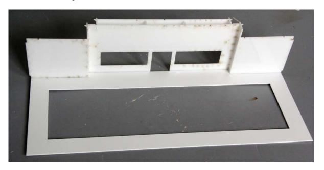
Glue the walls to the EDGE of the base plate, then continue with the side walls.
